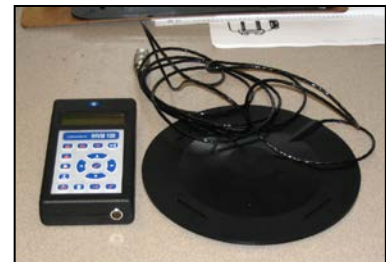
Vibration measurement device: the flat part goes on your seat
